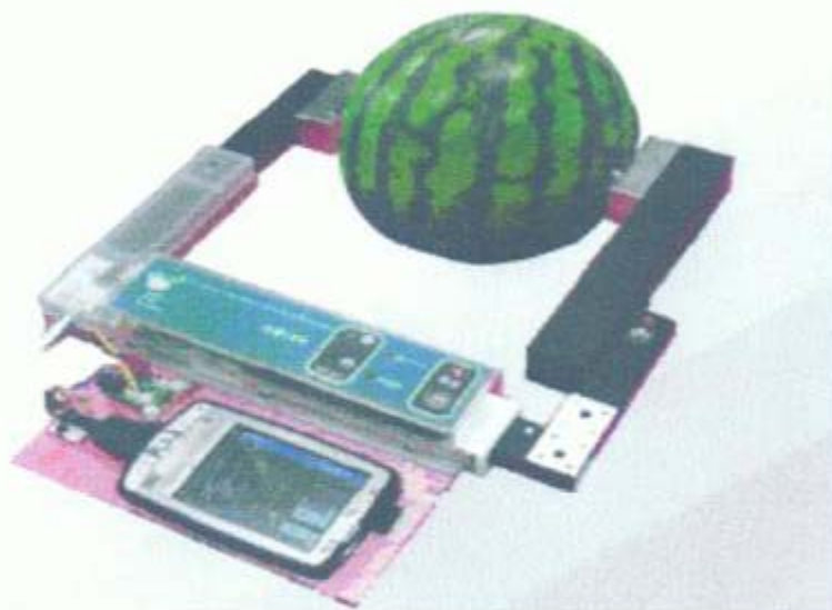
Fig. 5. A portable frequency response measurement instrument ( http://www.ava.co.jp )
